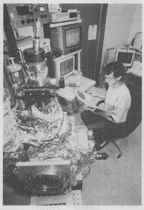
ATOM TRACKER — Brian Swartzentruber (1114) watches atoms move using the scanning tunneling microscope he modified to track individual atoms in rapid motion. (Photo by Mark Poulsen)
